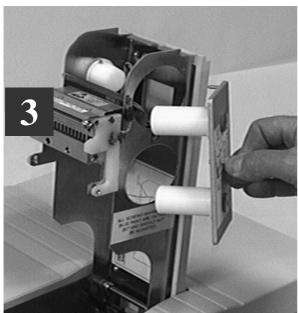
Open the Printer Cover by lifting the "Dzus" fastener ring and turning a quarter turn anti-clockwise. Remove the Dye Film carrier.
